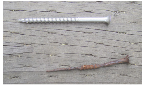
Here is an example of a rusted galvanized screw that was in the boardwalk and a stainless screw that will replace it.
